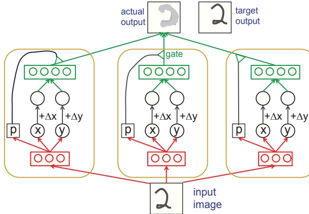
**Fig. 1.** Three capsules of a transforming autoencoder that models translations. Each capsule in the figure has 3 recognition units and 4 generation units.
